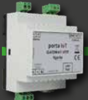
PORTA IOT 10020042 bidirectionele http gateway
